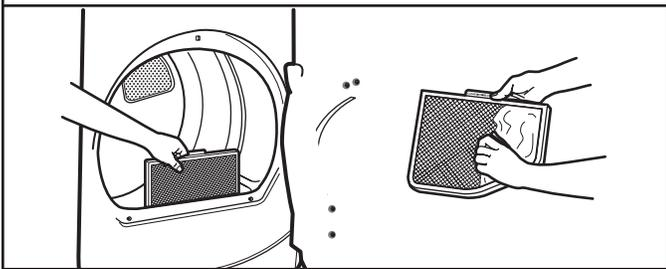
Clean the lint screen before each load. Pull the lint screen straight up. Roll lint off the screen with your fingers. Do not rinse or wash screen to remove lint. Wet lint is hard to remove. Push the lint screen firmly back into place.
